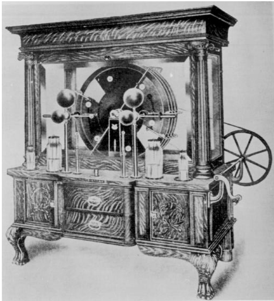
Fig. 1.1 Model of hand-operated Wimshurst friction generator
